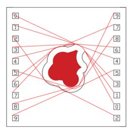
**Fig.7:** Deviated paths of the robots, when an irregularly curve shaped obstacle exists.
