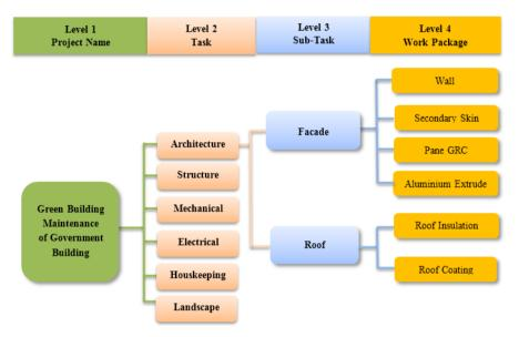
Fig. 4 WBS Details on Building Maintenance and repair of Green Buildings in Government Buildings
