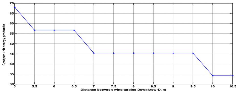
Fig. 6 Effect distance between turbine at a cost per unit energy
