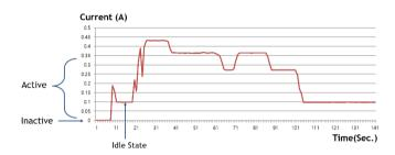
Fig 4. Active and Inactive State for TV
