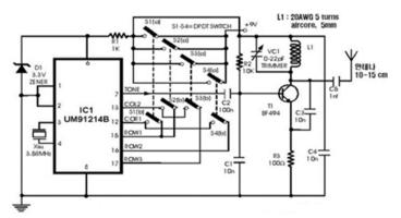
Fig. 4 Wireless transmit circuit schematic diagram
