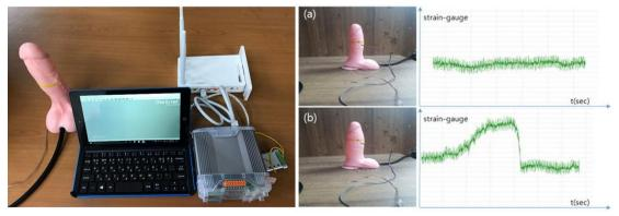
Fig. 8 Date graph of strain gauge achieved: (a) before erection (b) after erection
