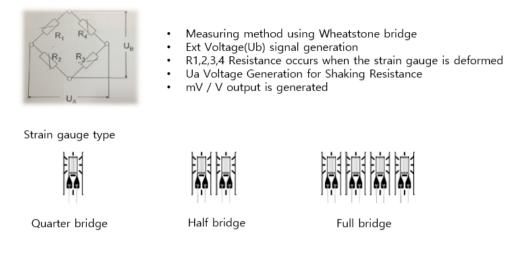
Fig. 2 Principle of strain gauge measurement
