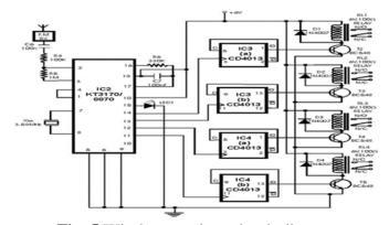
Fig. 5 Wireless receiver circuit diagram
