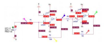
Fig. 3 Strain gauge schematic diagram
