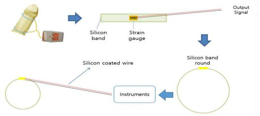
Fig. 1 Procedure for measuring data during tensile and compressing of strain gauge
