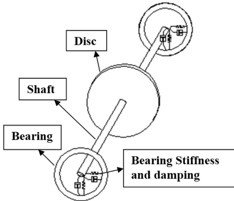
**Figure 2.** Rotor bearing system with stiffness and damping
