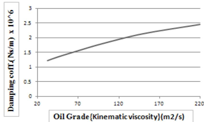
**Graph 4.** Damping coefficients variation with Oil viscosity
