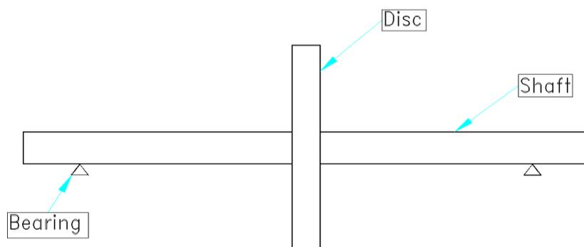
**Figure 1.** Simply Supported Rotor Bearing System
