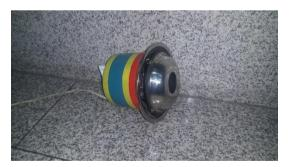
Fig 1. Portable Sound Fire Extinguisher
