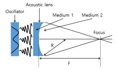
Fig 2. Schematic of Acoustic Lens
