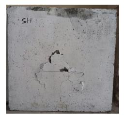
Fig.3 Failure pattern of solid HSC slab
