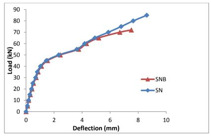
Fig.7 Load-deflection curve normal concrete slabs
