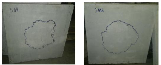
Fig.5 Failure pattern of solid MRPC slab Fig.6 Failure pattern of voided MRPC slab
