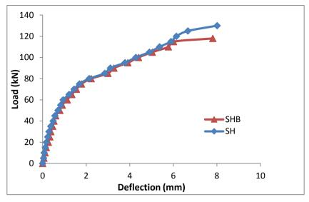
Fig.8 Load-deflection curve high strength concrete slabs
