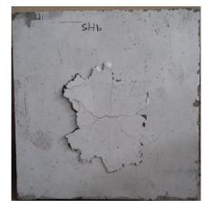
Fig.4 Failure pattern of voided HSC slab
