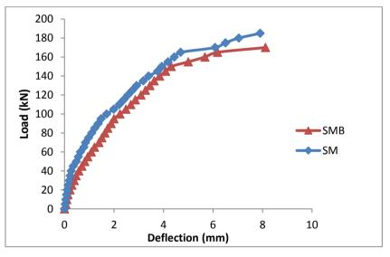
Fig.9 Load-deflection curve RPC slabs
