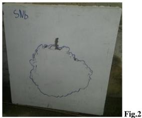
Failure pattern of voided normal concrete slab
