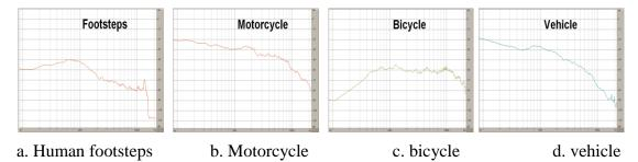
**Figure 6.** The natural frequency of the sound received from the microphone installed in the autonomous vehicle
