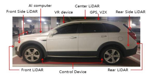
Figure 1. Principle of autonomous vehicle
