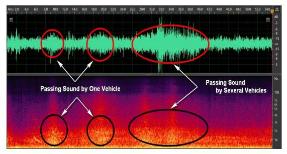
Figure 4. The sound Information on the driver's seat of the autonomous vehicle
