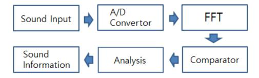
Figure 3. FFT diagram for obtaining sound information
