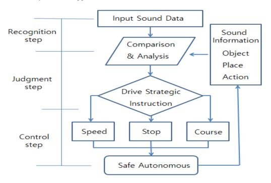
**Figure 7.** Flow chart of sound information technology application of autonomous driving car
