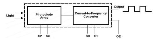
Fig.2: Functional block diagram of TCS3200
