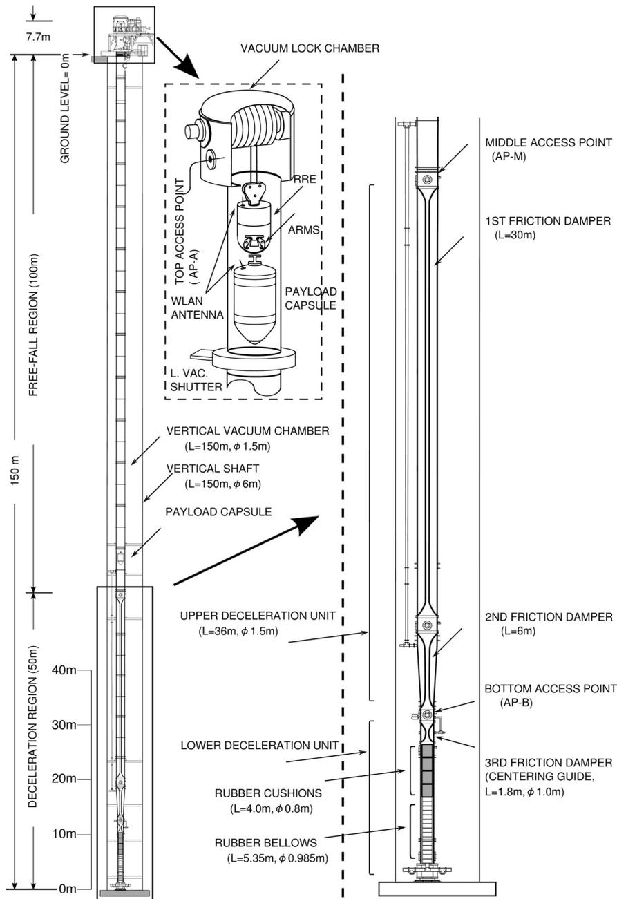
Figure 1: Schematic view of the microgravity experiment facility. The payload capsule is placed by the release-and-recovery equipment (RRE) at the top of the vertical vacuum chamber. Three friction dampers are shown. There are three access points (AP-A, AP-M and AP-B). The top access point (AP-A) is mounted on the viewing port in the vacuum lock chamber 5.5 m above ground level.
