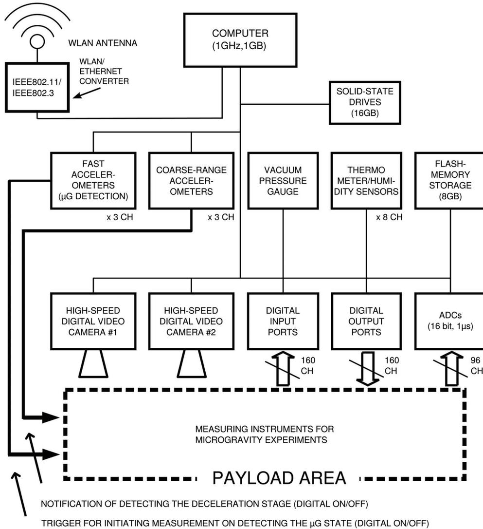
Figure 8: Schematic diagram of the payload capsule control system (PCCS) for the control and data acquisition (DAQ). The dashed box indicates the payload area where users can install their measuring instruments for their research purposes.
