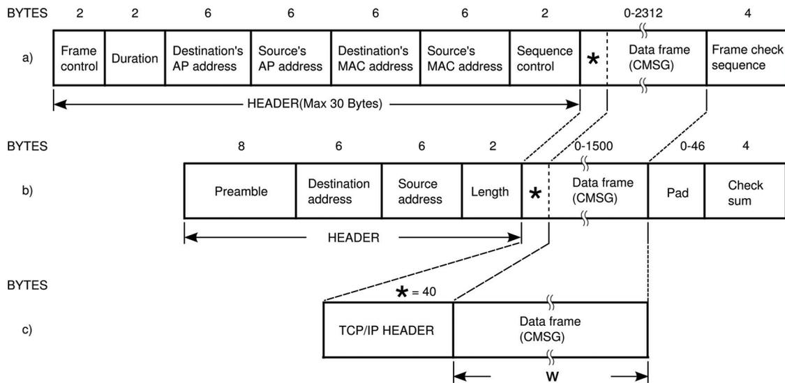
Figure 6: Formats of the data frame for the wireless network and Ethernet network. Each data frame consists of an embedded command message (CMSG) with a data length of  $w$  bytes; a) Format of the IEEE 802.11 data frame for wireless network (AP=physical address of an access point, MAC=medium-access-control defined in the standards). b) Format of the Ethernet data frame for IEEE 802.3 network. c) Simplified data structure of a TCP/IP datagram.
