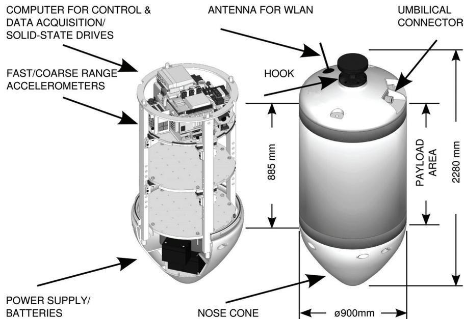
Figure 2: Structure of the payload capsule. The control equipment and communication device, including a computer, accelerometers, solid state disk drives and electronic interfaces for data acquisition, are installed at the top. An antenna for the wireless LAN (WLAN) is shown on the top cover.
