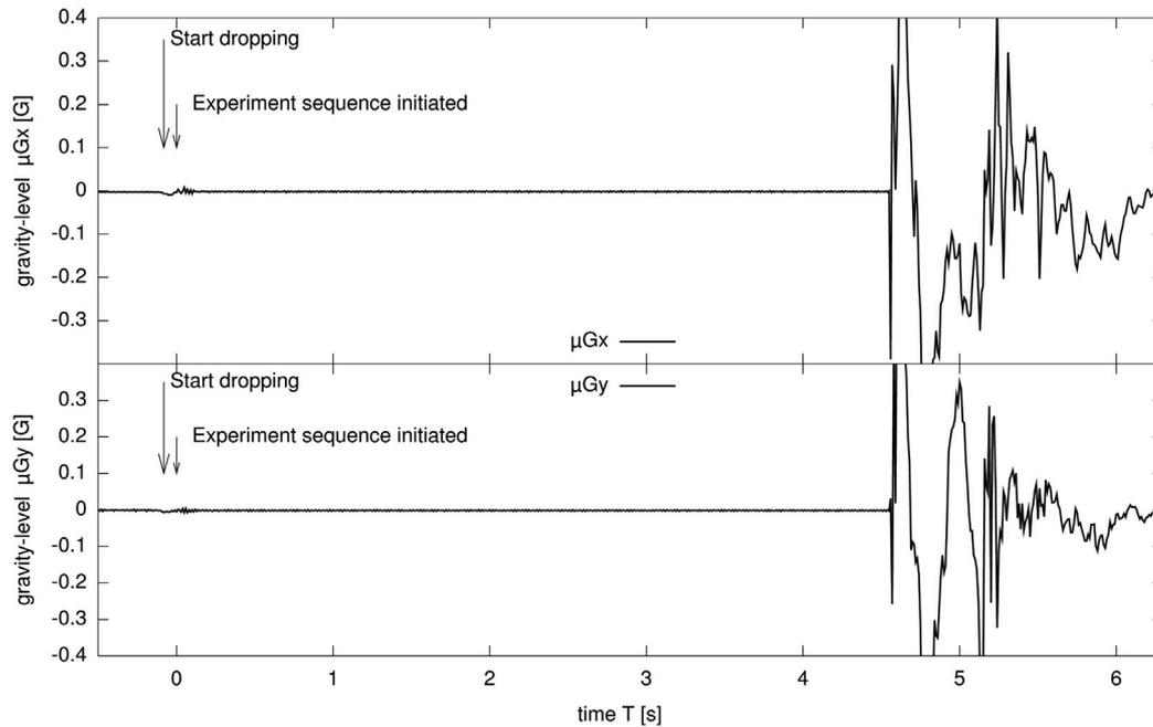
Figure 11: Typical horizontal gravity level traces measured by the system. (upper) x-component of the horizontal gravity  $\mu G_x$ . (lower) y-component of the horizontal gravity  $\mu G_y$ .
