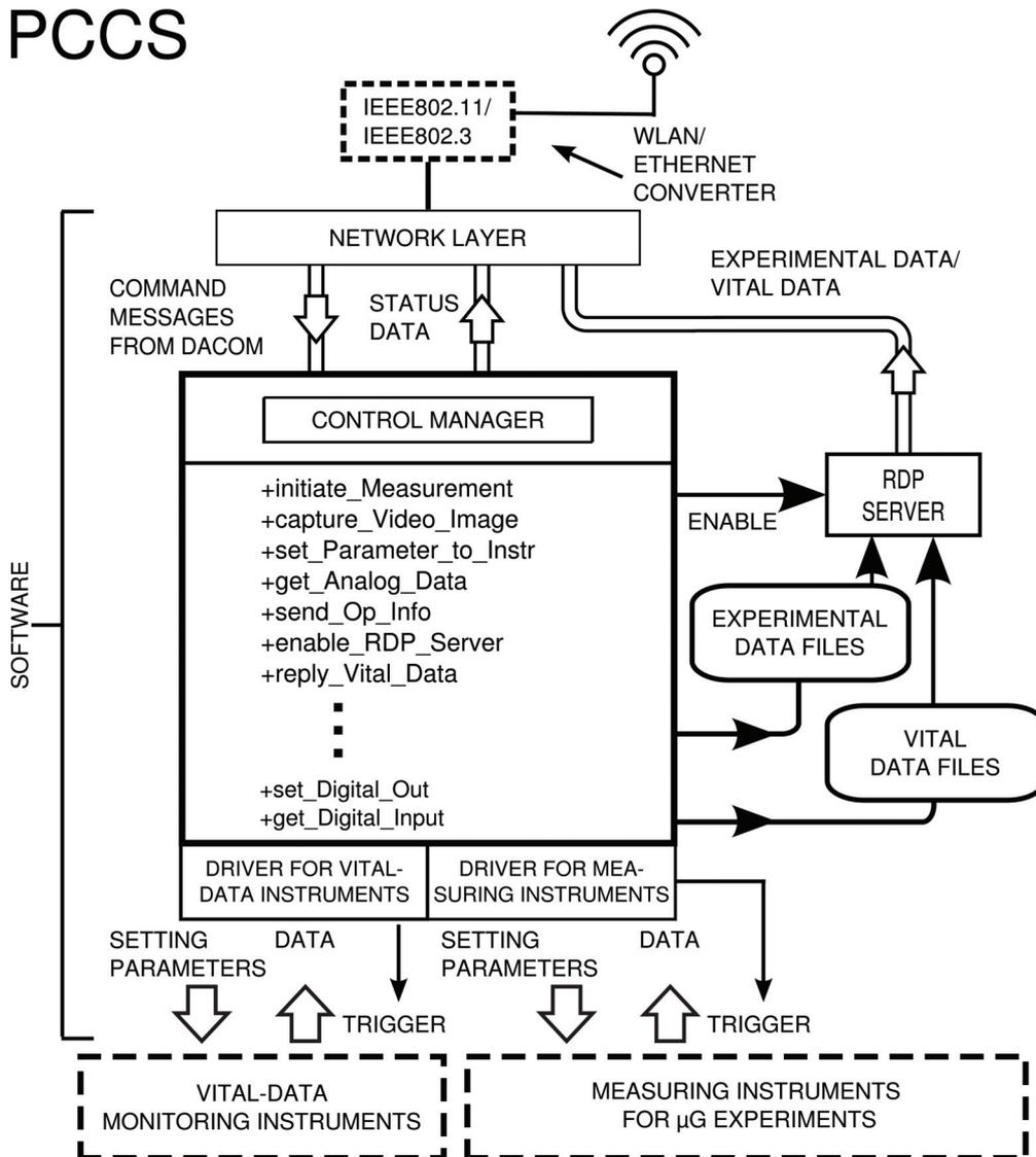
Figure 9: Schematic block diagram of the remote payload capsule control system (PCCS) showing the software (solid boxes) and hardware interfaces (dashed boxes) for the measuring instruments and vital-data monitoring instruments. The PCCS executes the command for the specified instrument in accordance with a preprogrammed sequence indicated by a '+' symbol.
