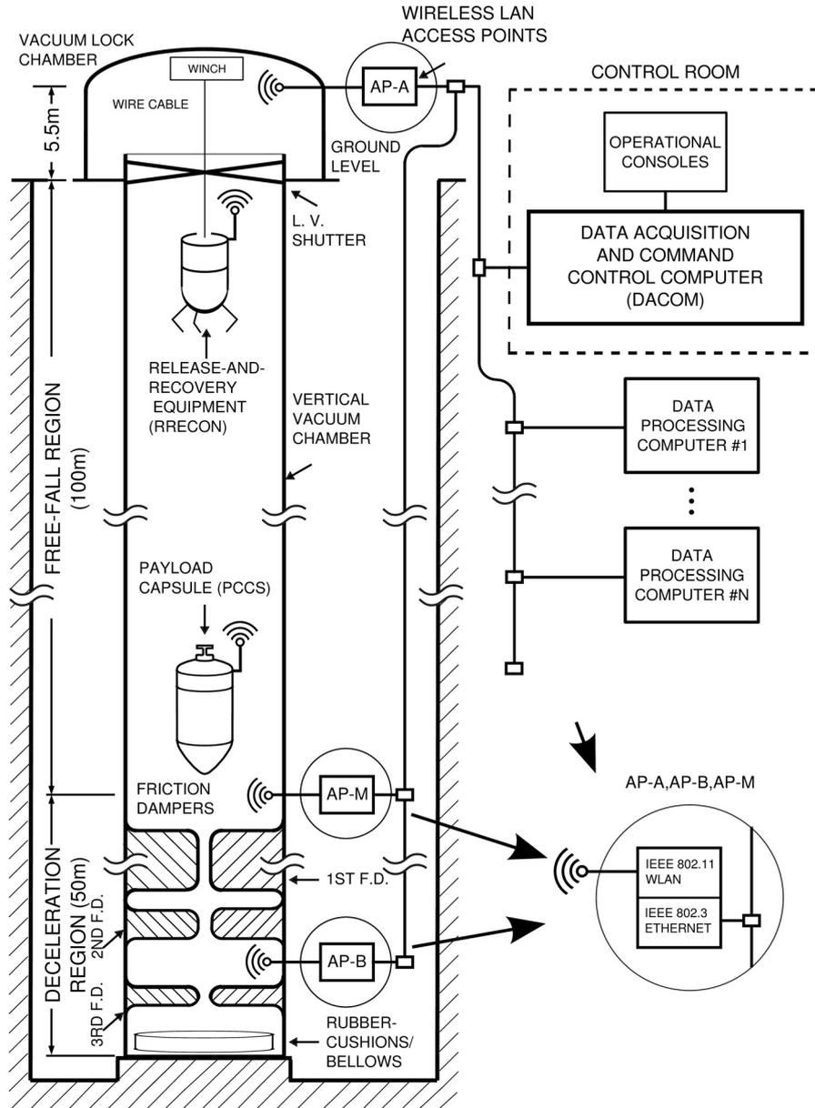
Figure 4: Schematic view of the microgravity experiment facility and the general configuration of the data acquisition and command control computer system for microgravity experiments.
