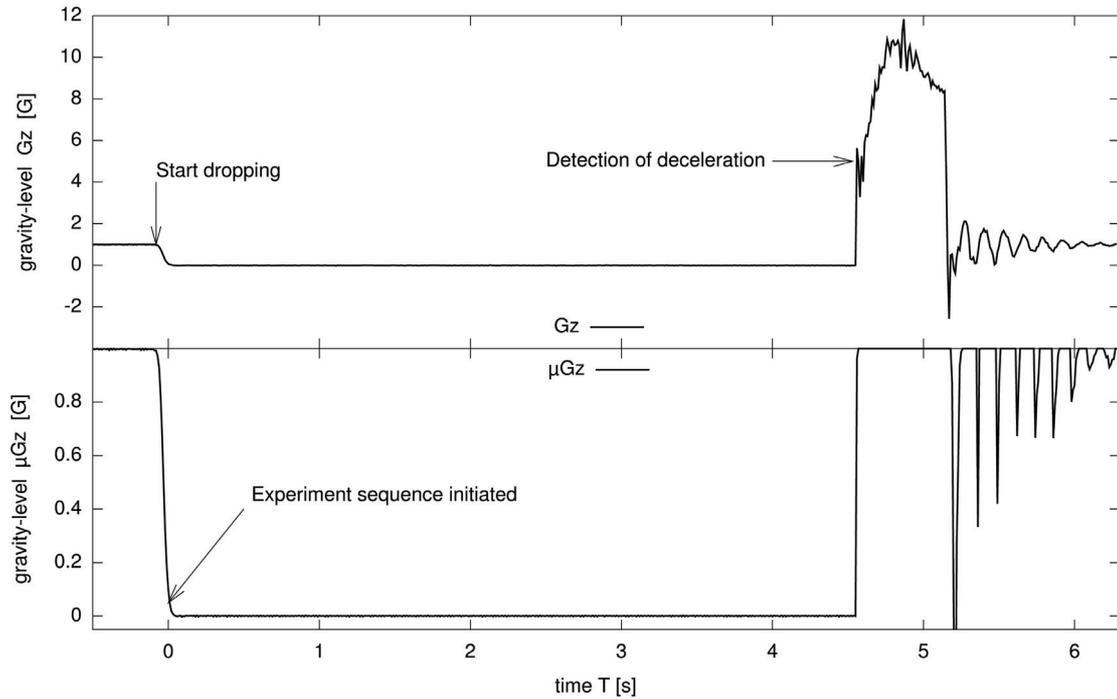
Figure 10: Typical vertical gravity level traces  $G_z$  measured by the system. (upper) Vertical gravity level  $G_z$  measured using the coarse-range accelerometer. (lower) Vertical gravity level  $\mu G_z$  measured by the fast-gravity accelerometer.
