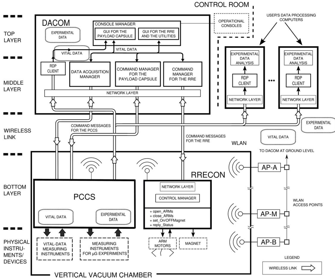
Figure 5: Schematic diagram of the software for the measuring and data acquisition system showing software (solid boxes) and hardware devices/instruments (dashed boxes). Command messages are delivered from the DACOM at ground level to the payload capsule control system (PCCS) and the remote controller for the RRE (RRECON) using the wireless link in the vertical vacuum chamber.
