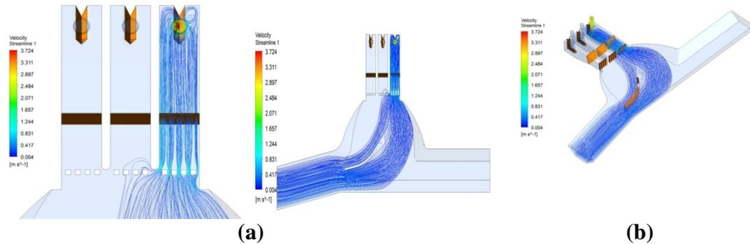
**Fig.6.1. Streamline plot for Case 5 modified Case 1 with Swirl Angles  $2.29^\circ$ ; (a) Plan View (b) 3D View**
