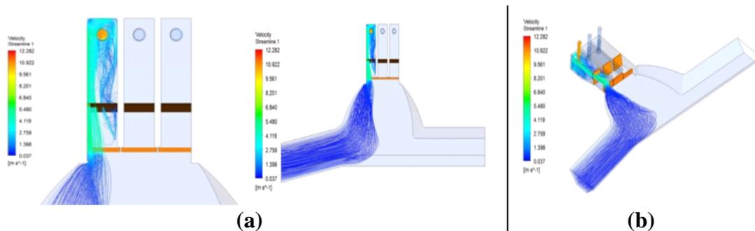
**Fig. 3.3** Streamline plot for Case 3 Pump 3 operate with Swirl Angles  $53.84^{\circ}$ ; (a) Plan View (b) 3D View
