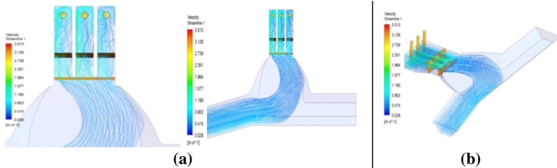
**Fig. 3.4 Streamline plot for Case 4 All Pumps operate with Swirl Angles 10.360, 21.430, and 15.230 respectively; (a) Plan View (b) 3D View**
