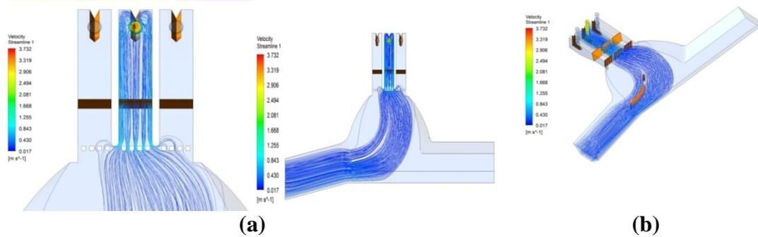
**Fig.6.2. Streamline plot for Case 6 modified Case 2 with Swirl Angles  $0.25^{\circ}$ ; (a) Plan View (b) 3D View**
