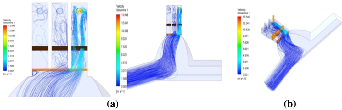
**Fig.3.1. Case 1 Pump 1 operate with Swirl Angles  $17.84^\circ$ ; (a) Plan View (b) 3D View**
