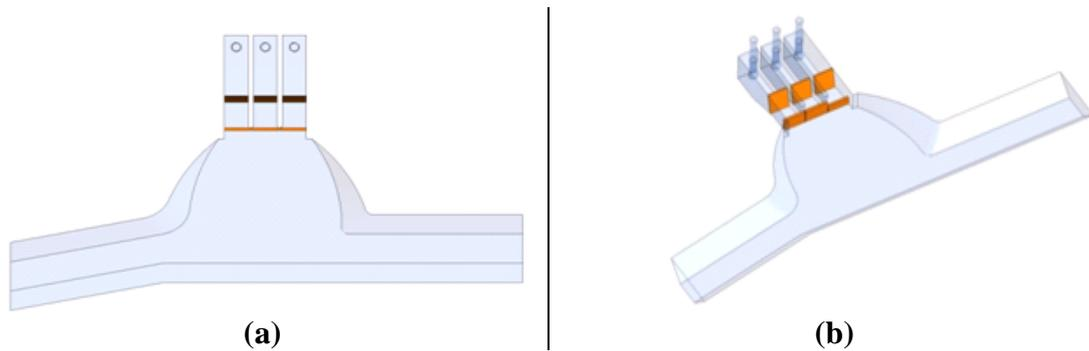
**Fig.1. Initial Sump Geometry used for CFD analysis; (a) Plan View (b) 3D View**
