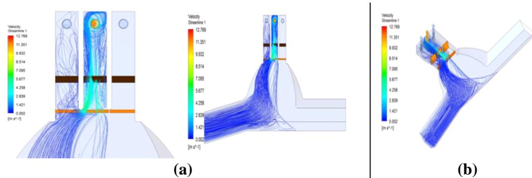
**Fig. 3.2** Streamline plot for Case 2 Pump 2 operate with Swirl Angles  $35.81^{\circ}$ ; (a) Plan View (b) 3D View
