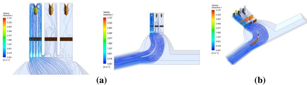
**Fig.6.3. Streamline plot for Case 7 modified Case 3 with Swirl Angles  $0.25^{\circ}$ ; (a) Plan View (b) 3D View**
