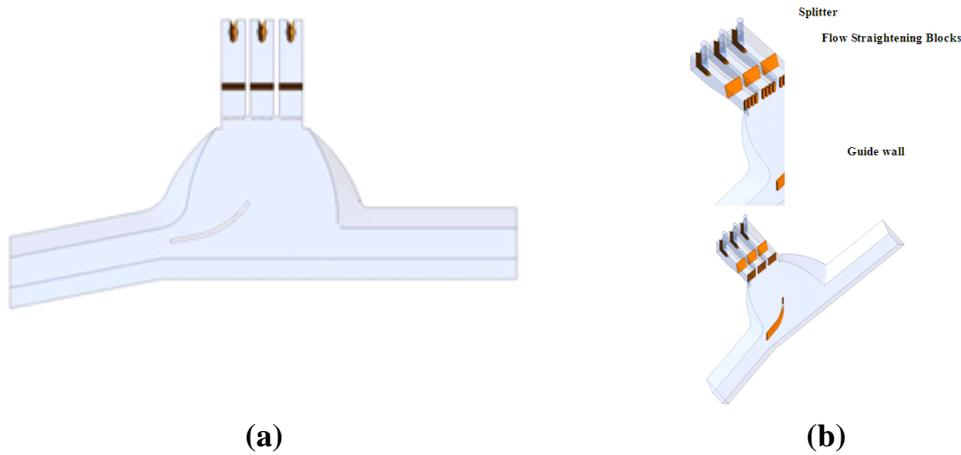
**Fig.4. Modified Sump Geometry for CFD analysis; Plan View (b) 3D View**
