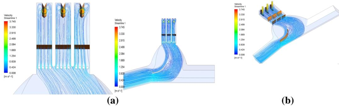
**Fig.6.4. Streamline plot for Case 8 modified Case 4 with Swirl Angles  $0.25^{\circ}$ ; (a) Plan View (b) 3D View**
