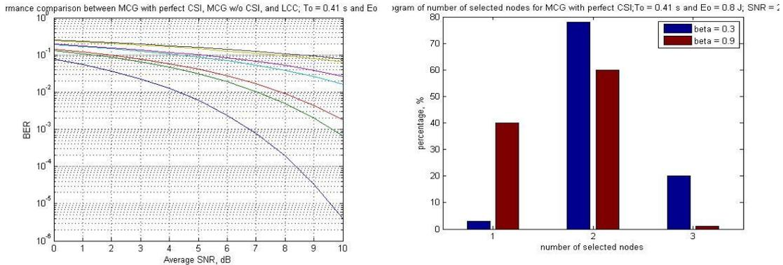
**Fig. 5:** Performance comparison between MCG with perfect CSI, MCG w/o CSI, and LCC;  $T_o = 0.41$  s and  $E_o = 0.8$  J. **Fig. 6:** Histogram of number of selected nodes for MCG with perfect CSI;  $\square\square = 0.41$ s and  $\square\square = 0.8$  J; SNR = 22.4 dB.
