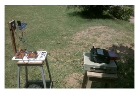
Fig. 2: Designed working Prototype of solar tracker.
