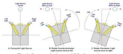
Fig. 1: Concept of using two LDRs for sensing.
