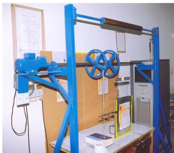
**Fig. 1:** Picture of thin film coating set-up by solgel dip coating process.
