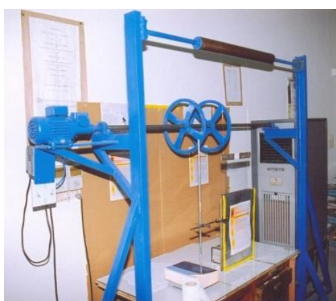
Fig. 1: Picture of thin film coating set-up by solgel dip coating process.
