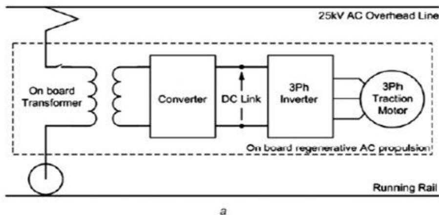
**Fig.4.** Block diagram of AC locomotive
