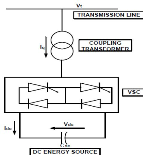
**Fig.6** Structure of STATCOM
