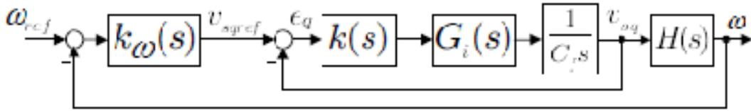
**Fig. 5. Block diagram of the frequency control loop**
