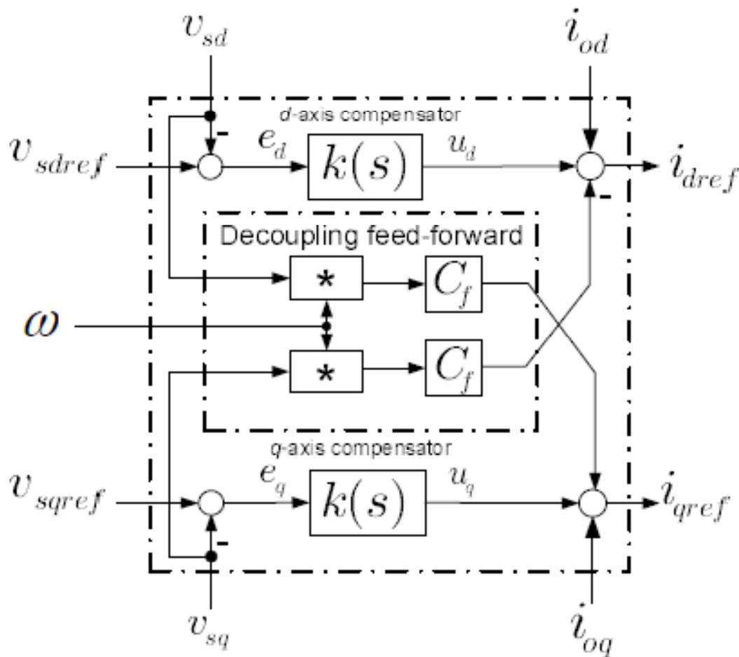
**Fig. 3. Block diagram of the voltage control**
