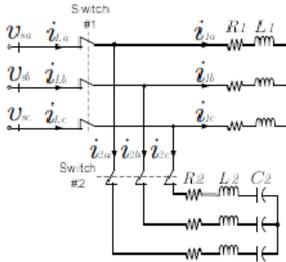
Fig. 7. Schematic diagram of the configurable passive load
