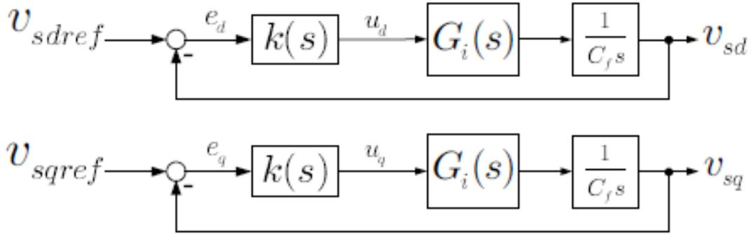
**Fig. 4. Equivalent block diagram for the closed –loop voltage control scheme**
