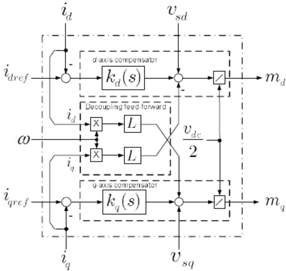
**Fig. 2. Block diagram of the current-control scheme**
