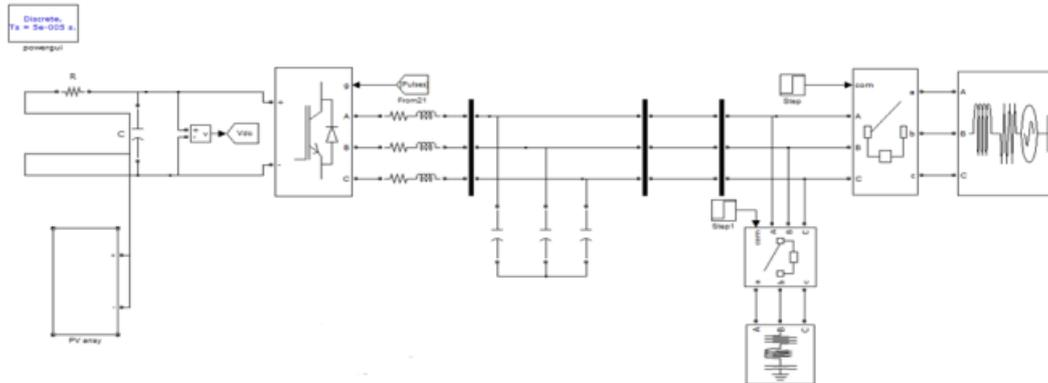
**Fig. 14. simulink model of the electronically-interfaced Distributed Resource (DR) unit in the islanded mode**
