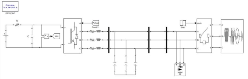
**Fig. 6. Simulink model of the electronically-interfaced Distributed Resource (DR) unit in the islanded mode**
