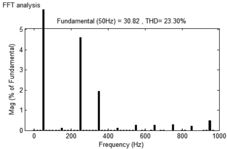
Fig.11. Harmonic Spectrum with  $m_a=1$  by using COPWM control technique
