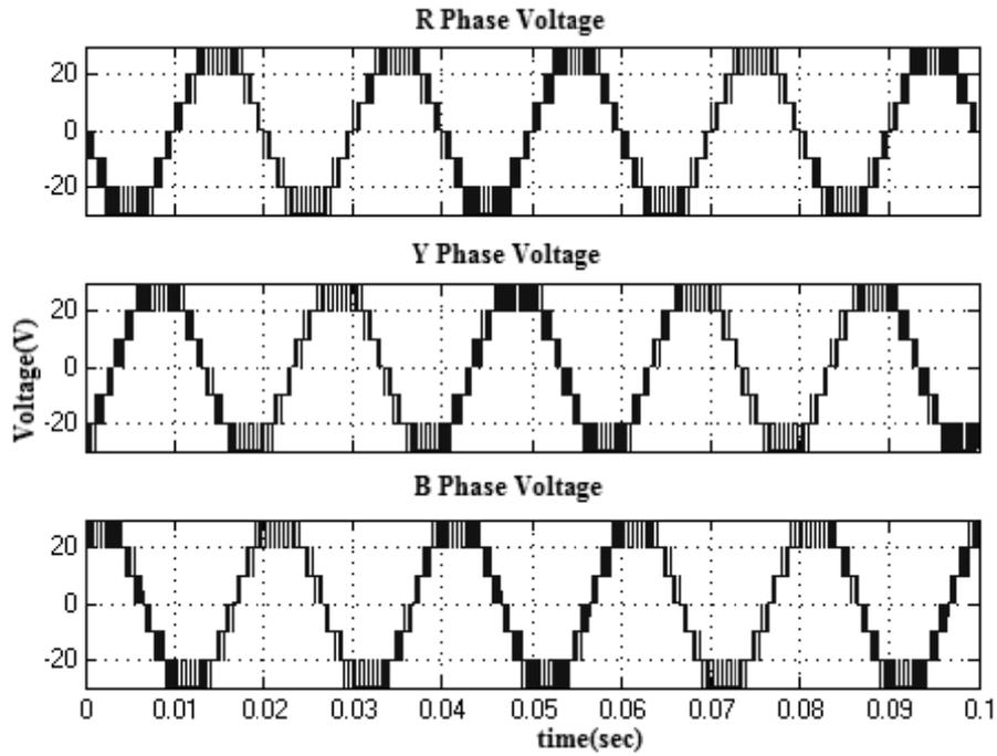
Fig.10. Output Voltage generated by PD PWM control strategy
