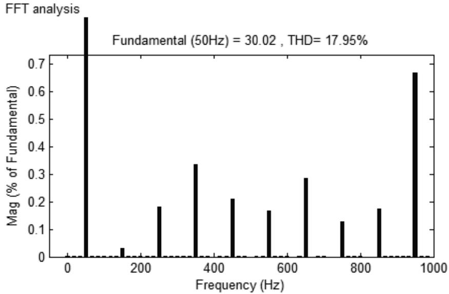
Fig.14. Harmonic Spectrum with  $m_a=1$  by using APOD PWM control technique
