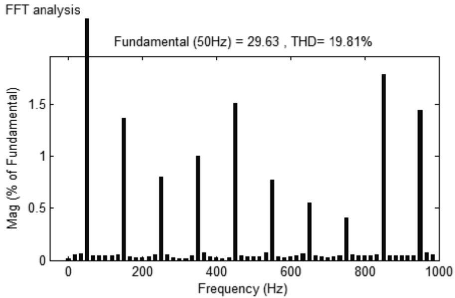
Fig.12. Harmonic Spectrum with  $m_a=1$  by using IS PWM control technique
