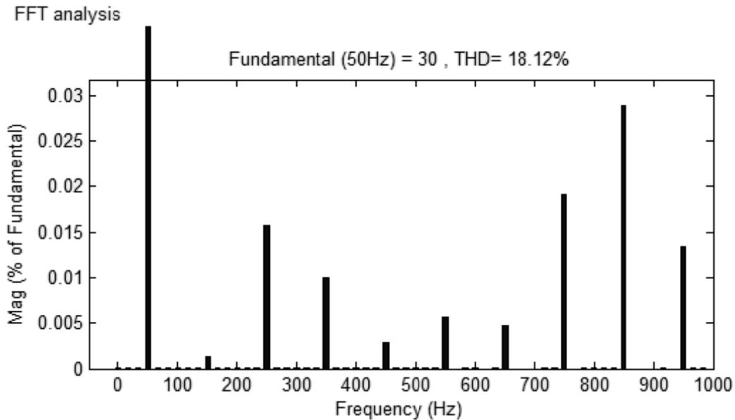
Fig.13. Harmonic Spectrum with  $m_a=1$  by using APOD PWM control technique
