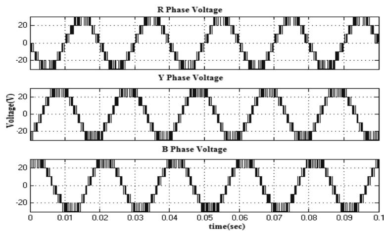
Fig.9. Output Voltage generated by APOD PWM control strategy
