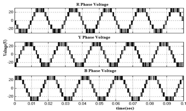
Fig.8. Output Voltage generated by IS PWM control strategy
