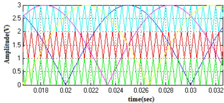
Fig.5. APOD PWM waveform
