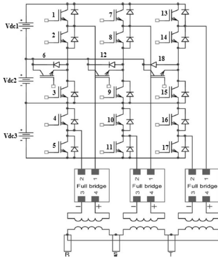
Fig.2. Three-phase Reverse Voltage MLI circuit
