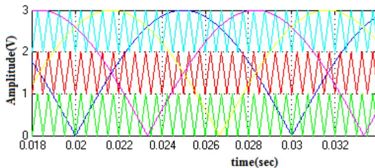
Fig.6. PD PWM waveform
