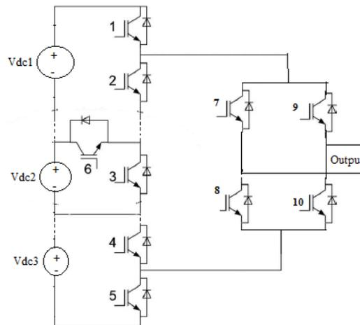
Fig.1. Reverse Voltage MLI circuit
