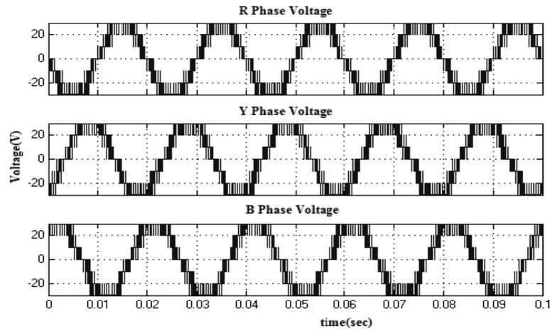
Fig.7. Output Voltage generated by CO PWM control strategy
