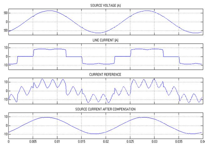
Figure 7. Source current for Phase C after compensation
