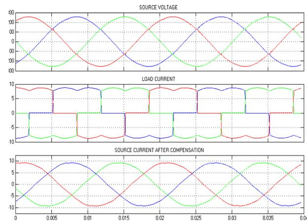
Figure 8.Source Current After compensation
