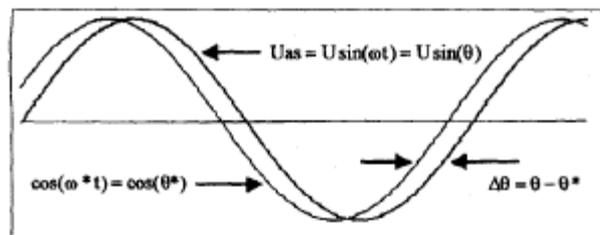
**Figure 3. Input phase voltage and PLL output**
