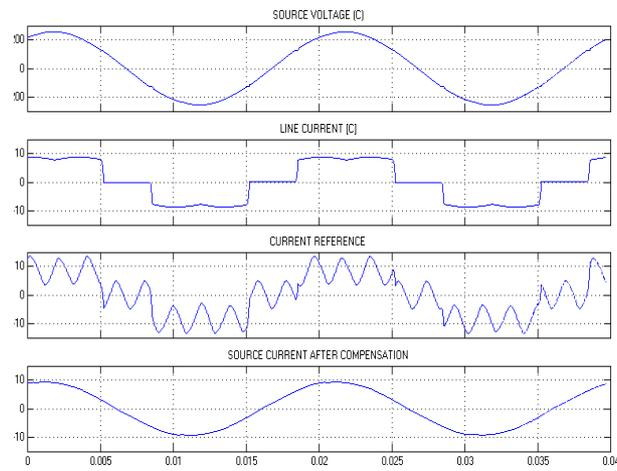
Figure 5. Source current for Phase A after compensation
