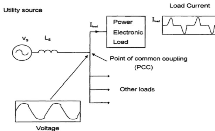
Figure 1. Harmonic distortion at PCC
