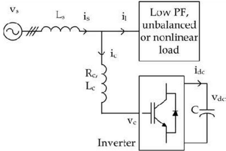
Figure 2. Basic Compensation principle
