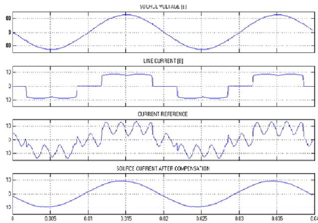
Figure 6. Source current for Phase B after compensation
