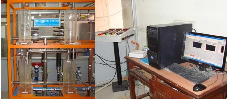
**Figure 2:** Experimental setup of the quadruple-tank process.
