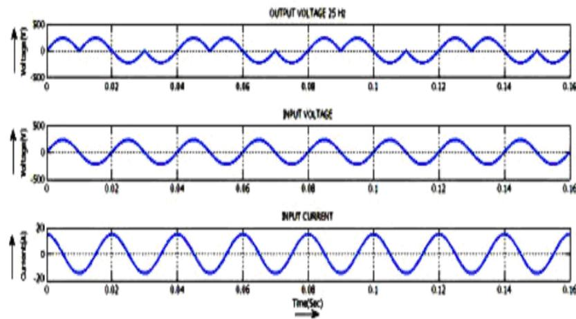
**Figure 8:** Input current and input voltage for 50 Hz and output voltage for 25 Hz
