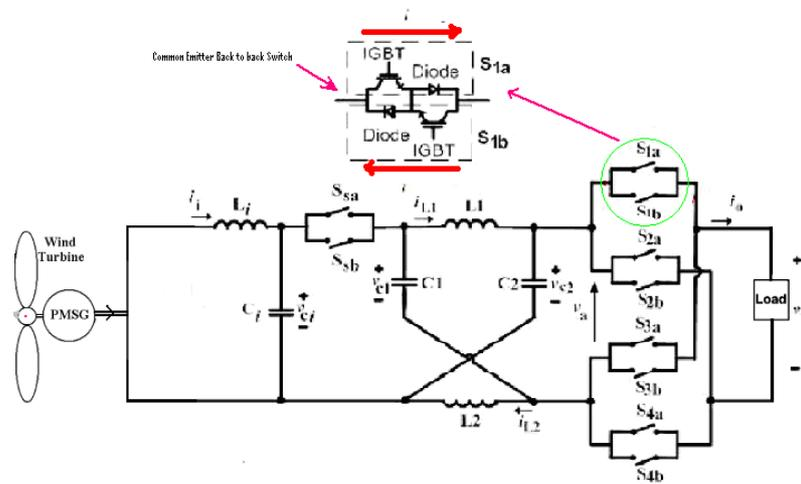
Figure 3: Proposed single-phase Z-source matrix Converter topology
