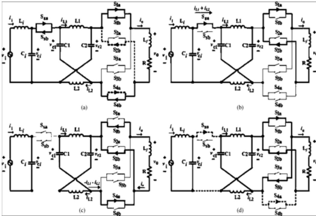
**Figure 6:** Stage 1 for the boost mode for a frequency of 100 Hz. (a) State 1. (b) Commutation state when  $iL_1 + iL_2 + i_o > 0$  (c) Commutation state when  $-iL_1 - iL_2 + i_o > 0$  (d) State 2.
