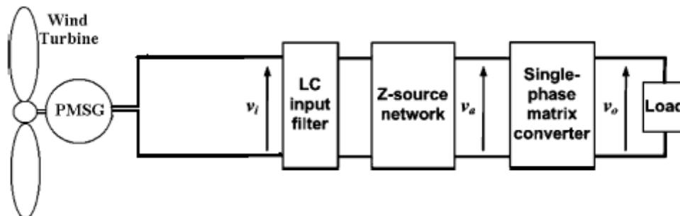
**Figure 2:** General Block diagram of the proposed Topology.
