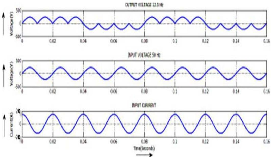
**Figure 7:** Input current and input voltage for 50 Hz and output voltage for 12.5 Hz.
