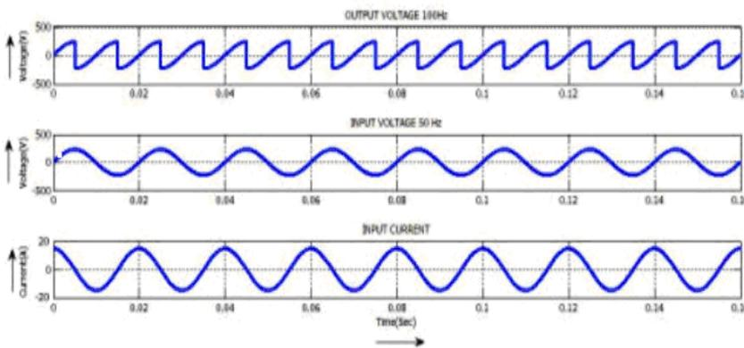
**Figure 10:** Input current and input voltage for 50 Hz and output voltage for 100 Hz
