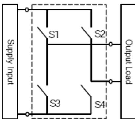
Figure 4: SPMC circuit configuration
