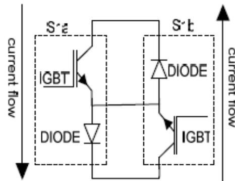
Figure 5: Bi-directional switch module (common emitter configuration)
