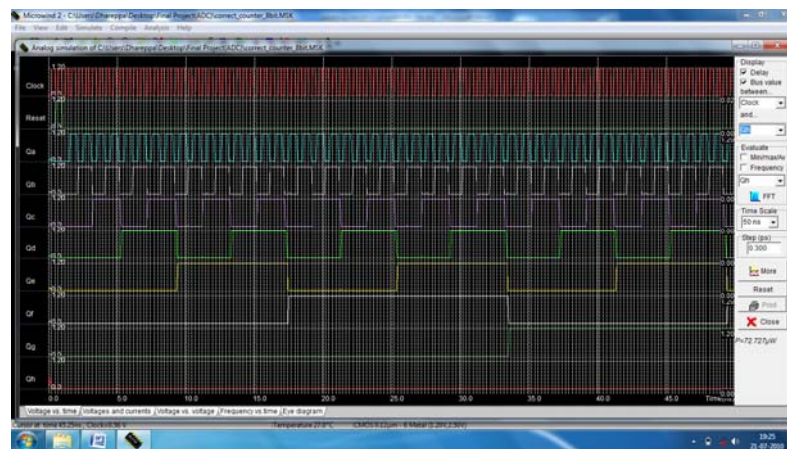
Figure 5: The simulation result of the 8-bit asynchronous binary counter.
