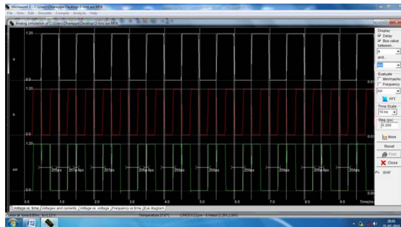
Figure 3: Simulation result of a 4T-XOR Gate.
