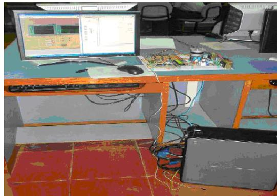
**Figure 4:** Experimental Setup for speed control using Labview.
