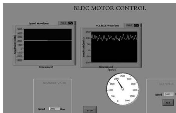
**Figure 5:** Voltage waveform and Speed for set speed of 2000 rpm.
