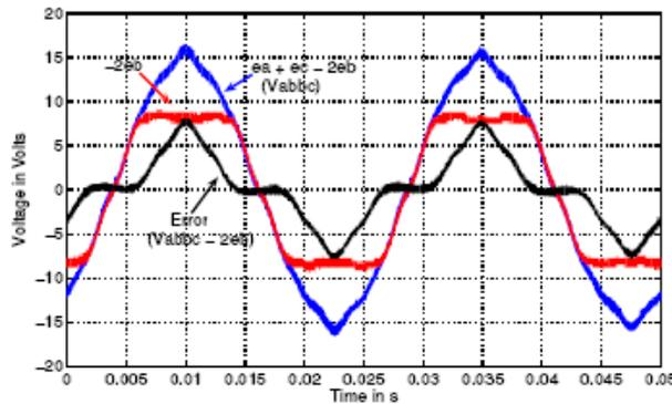
**Figure 2:** Line voltage difference and back –EMF.
