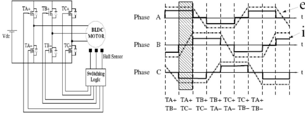
**Figure 1:** PMBLDC drive and typical phase current and back-EMF waveform.
