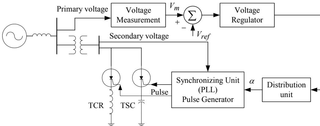
**Figure 1:** Single-line diagram of a Static Var Compensator and its control system.
