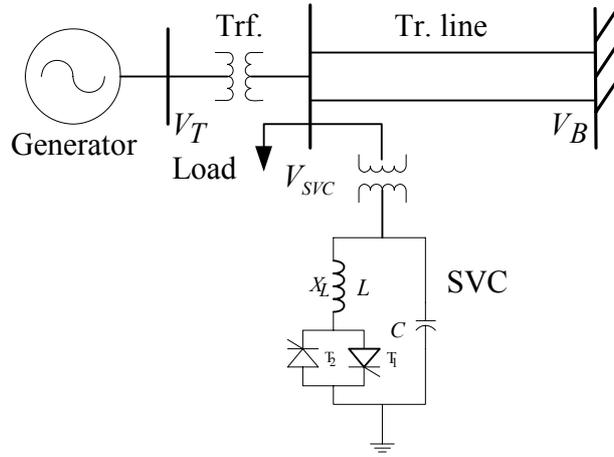
**Figure 6:** Single-machine infinite-bus power system with SVC.
