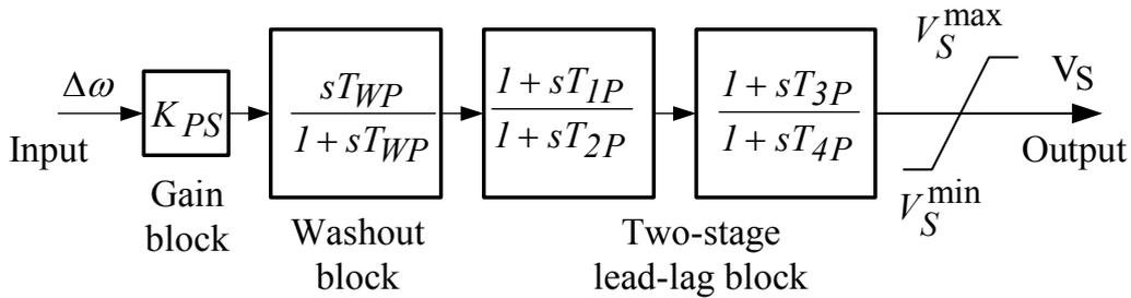
**Figure 3:** Structure of the power system stabilizer.
