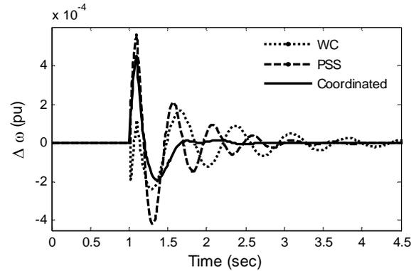
Figure 17: Speed deviation response for Case-IV.
