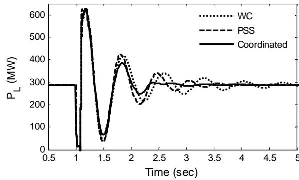
**Figure 8:** Tie-line power flow response for Case-I.
