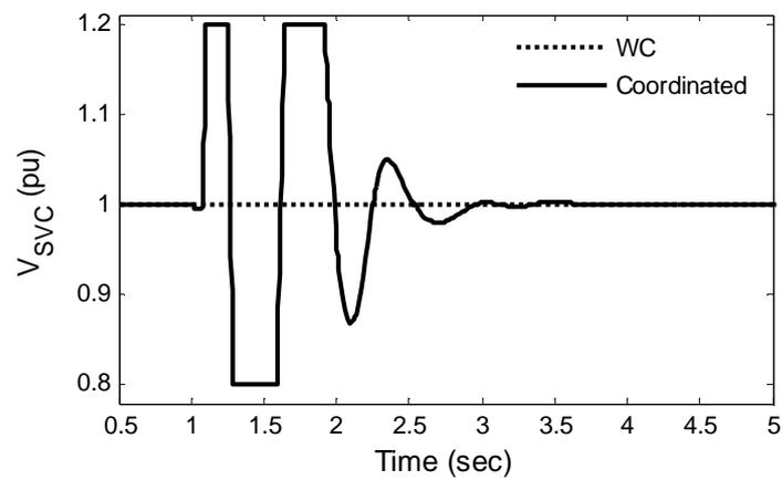
**Figure 16:** SVC reference voltage signal for Case-III.
