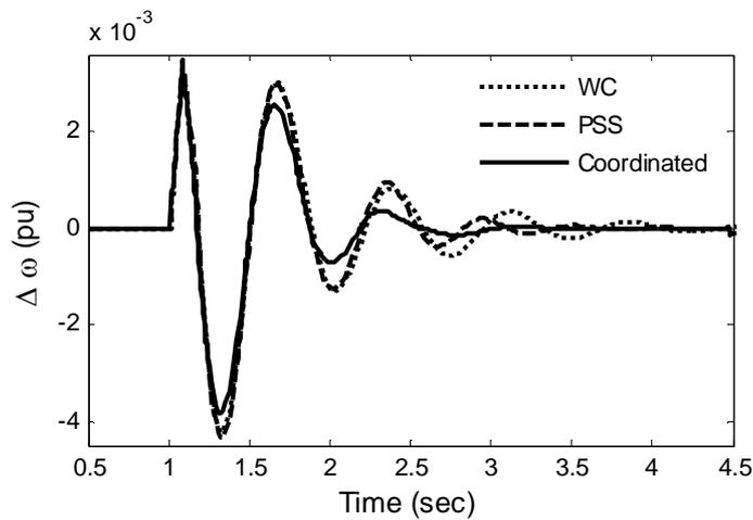
Figure 11: Speed deviation response for Case-II.
