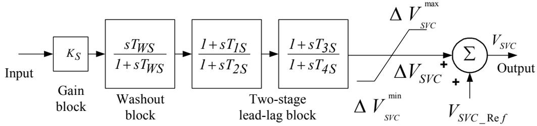
**Figure 2:** Structure of the SVC-based controller.
