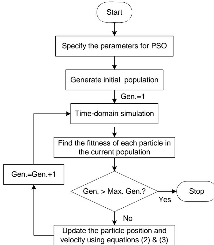
**Figure 5:** Flowchart of particle swarm optimization algorithm.
