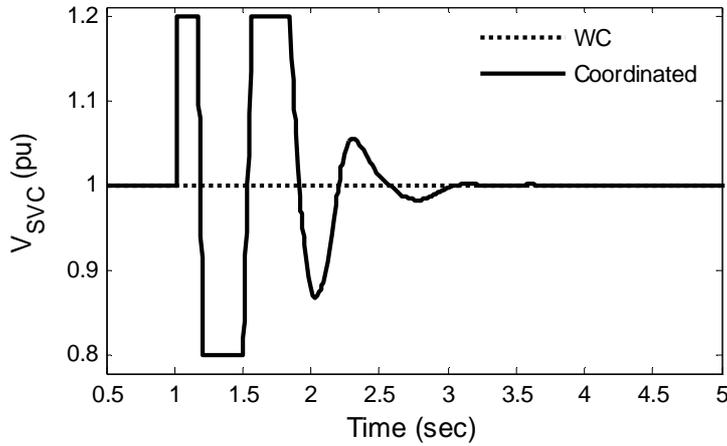
Figure 10: SVC reference voltage signal for Case-I.
