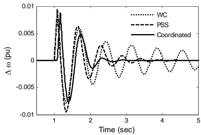
**Figure 14:** Speed deviation response for Case-III.
