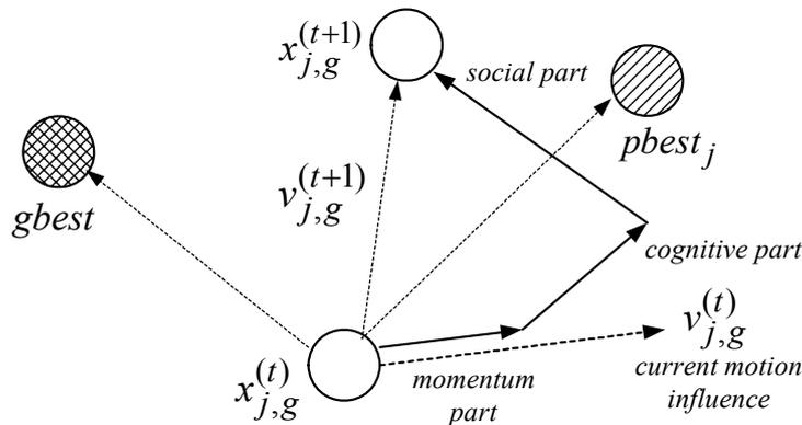
**Figure 4:** Description of velocity and position updates in particle swarm optimization technique.
