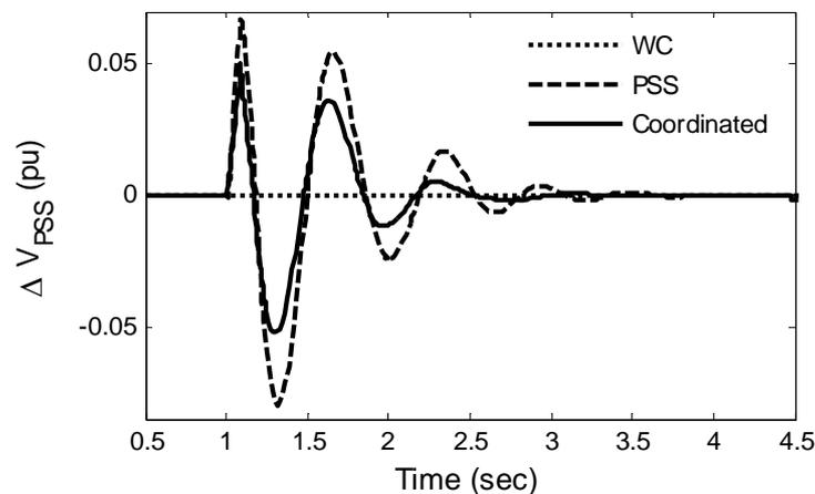
**Figure 12:** Stabilising signal of PSS for Case-II.
