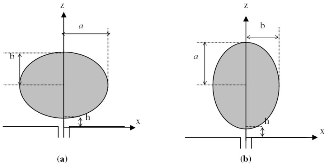
**Figure 2:** a) Elliptical disc monopole fed along minor axis, b) elliptical disc monopole fed along major axis.
