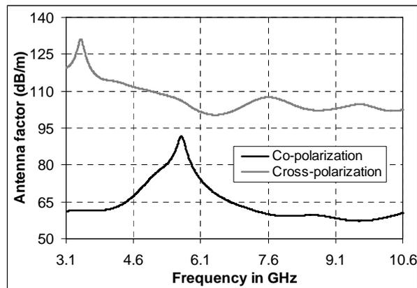
**Figure 11:** Plot of antenna factor versus frequency of truncated triangular monopole antenna.
