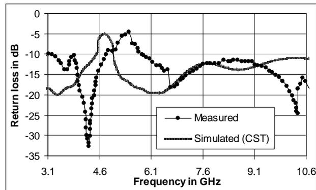
**Figure 4:** Plot of return loss versus frequency of band-notched circular ring monopole antenna with stub [12].
