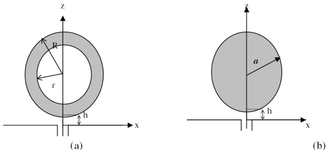
**Figure 1:** a) Configuration of annular circular monopole, b) circular disc monopole.
