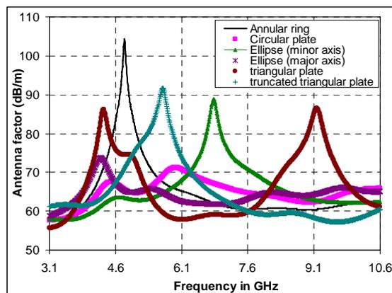
**Figure 12:** Plot of antenna factor versus frequency of different planar monopole antennas.
