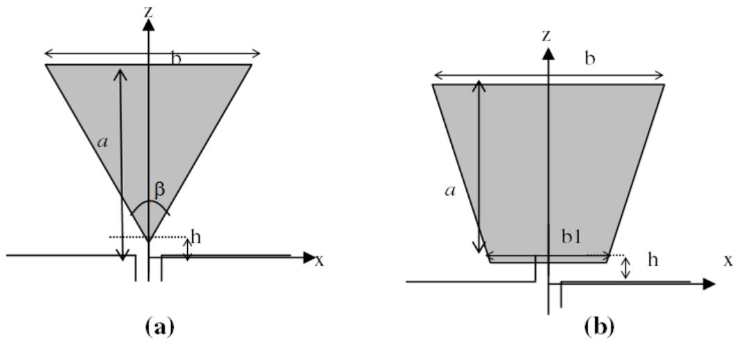
**Figure 3:** a) Configuration of planar triangular monopole antenna, b) Configuration of truncated equilateral triangular monopole antenna.
