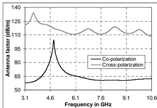
**Figure 6:** Plot of antenna factor versus frequency of annular circular monopole antenna.
