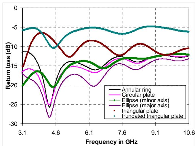
**Figure 5:** Plot of return loss versus frequency of different planar monopole antennas.
