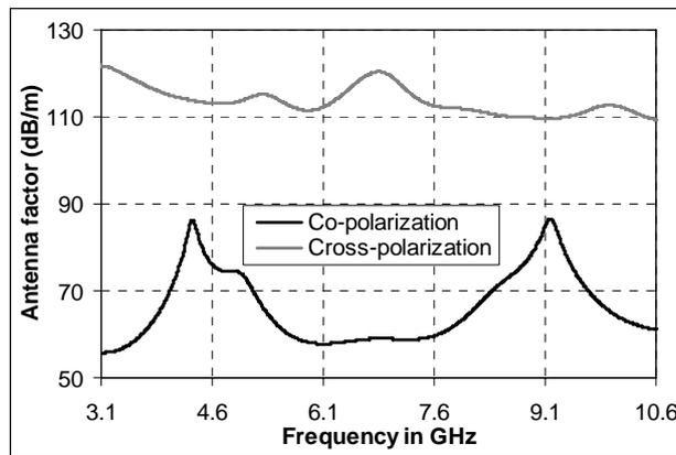
**Figure 10:** Plot of antenna factor versus frequency of triangular monopole antenna.
