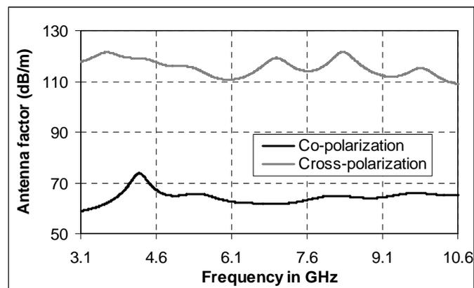
**Figure 9:** Plot of antenna factor versus frequency of elliptical disc monopole antenna fed along major axis.
