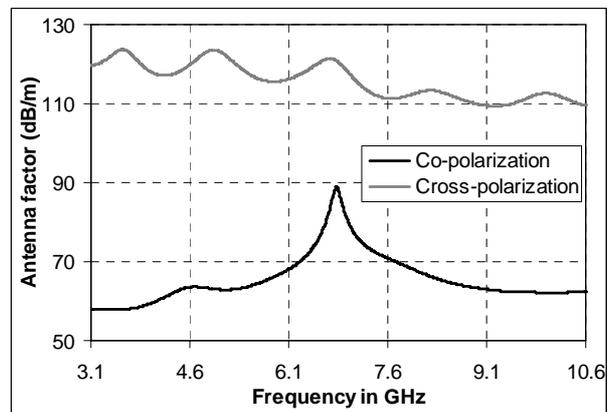
**Figure 8:** Plot of antenna factor versus frequency of elliptical disc monopole antenna fed along minor axis.
