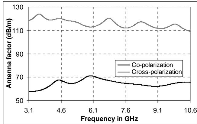
**Figure 7:** Plot of antenna factor versus frequency of circular monopole antenna.
