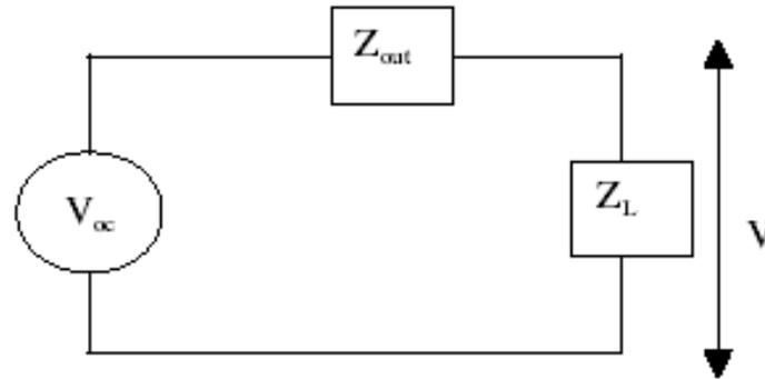
**Figure 3:** Equivalent circuit diagram of an antenna used as EMI sensor [3].
