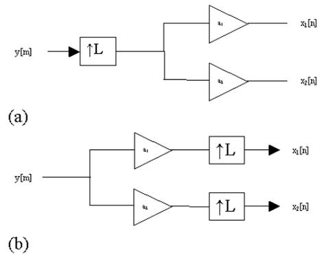
Figure 10(a) & (b): Block diagram of 4<sup>th</sup> Identity
