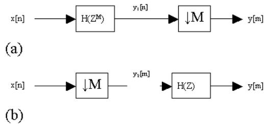
Figure 9(a) & (b): Block diagram of 3<sup>rd</sup> Identity
