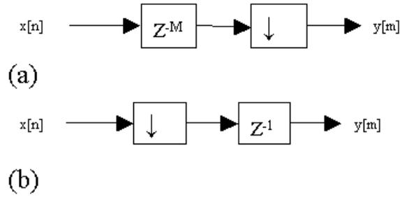
Figure 8(a) & (b): Block diagram of 2<sup>nd</sup> Identity
