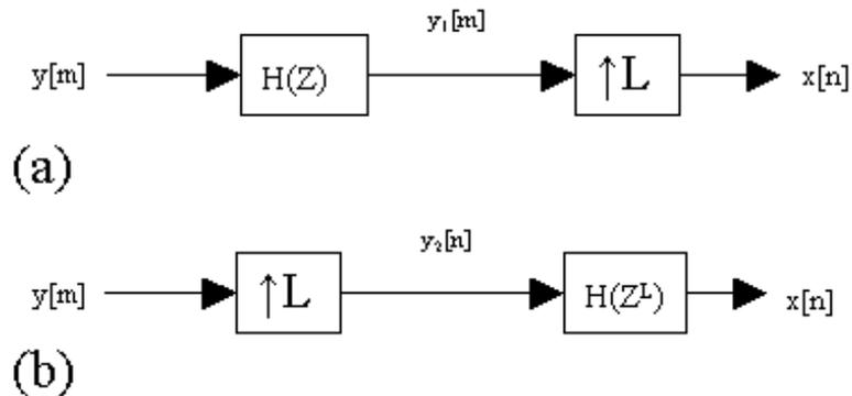
**Figure 12(a) & (b):** Block diagram of 6<sup>th</sup> Identity
