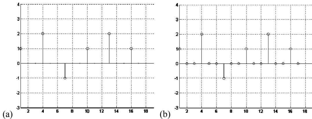
**Figure 5:** Up-sampling process (a) Original Signal (b) Increasing the sampling rate by inserting zero between the original samples
