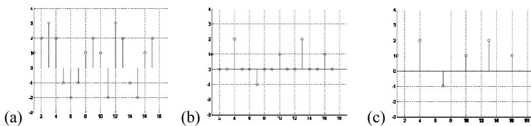
**Figure 2:** Down-sampling as a two step process (a) Original Signal (b) Replacing the  $M-1$  samples with zero samples at  $M=3$  (c) Removing the zero samples to reduce the sampling rates
