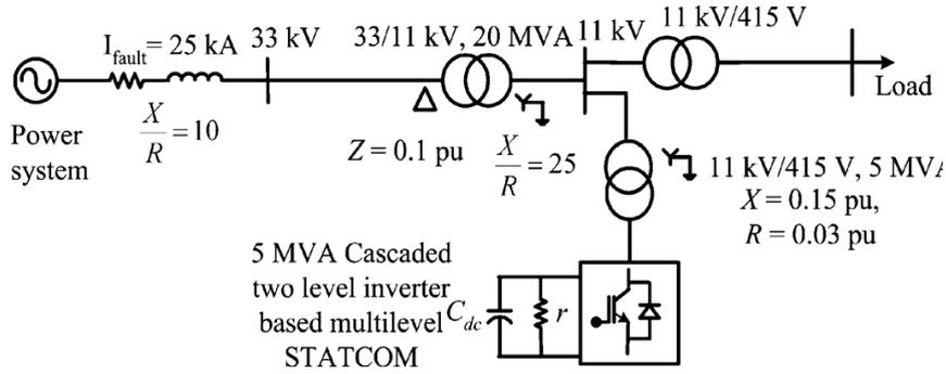
**Fig.1:** Power system and the STATCOM model
