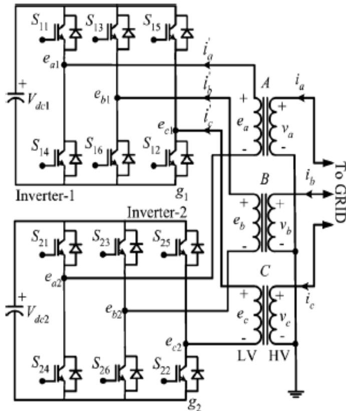
**Fig.2:** Cascaded two-level inverter based multilevel STATCOM
