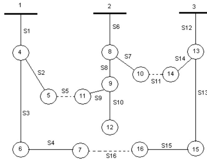
**Figure 1 :** Single Line Diagram Of Ieee 16-Bus System
