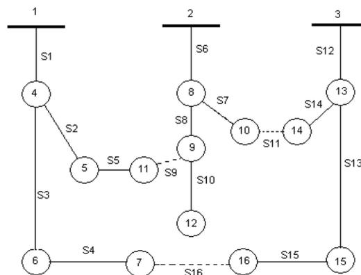
**Figure 4 :** Example Problem's Result After Applying Prim's Algorithm
