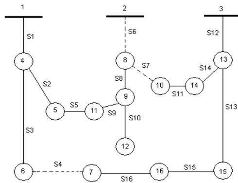
**Figure 5 :** Result of IEEE 16–bus system for a outage at line S6
