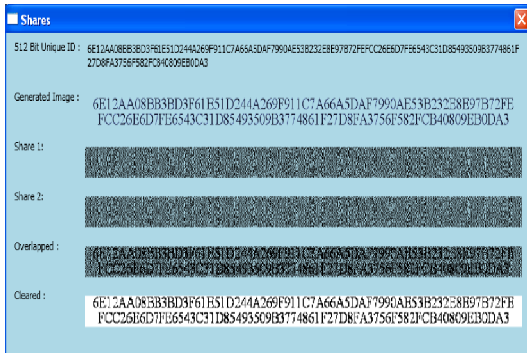
Figure 3. Screenshot of a Window that shows how a 512 bit random number is made into share 1 & share 2. Overlapping of shares is also shown in the figure.
