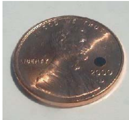
Figure 5.1: The dot above the date on this penny is the full size of the artificial silicon retina.
