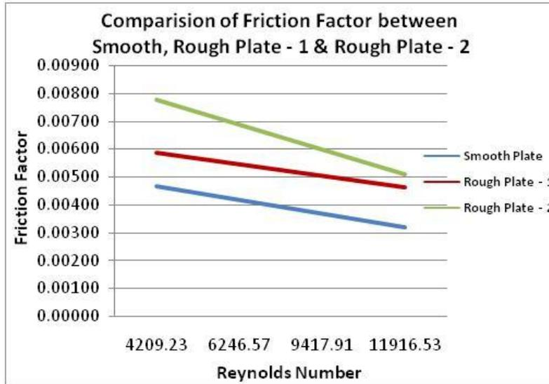
**Fig. 3** Reynolds Number Vs Friction Factor
