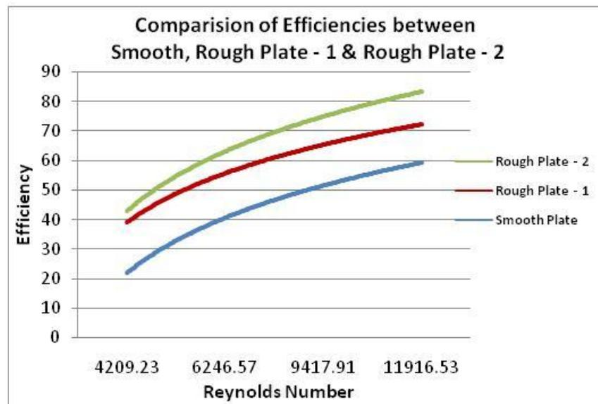
**Fig. 2** Reynolds Number Vs Efficiency
